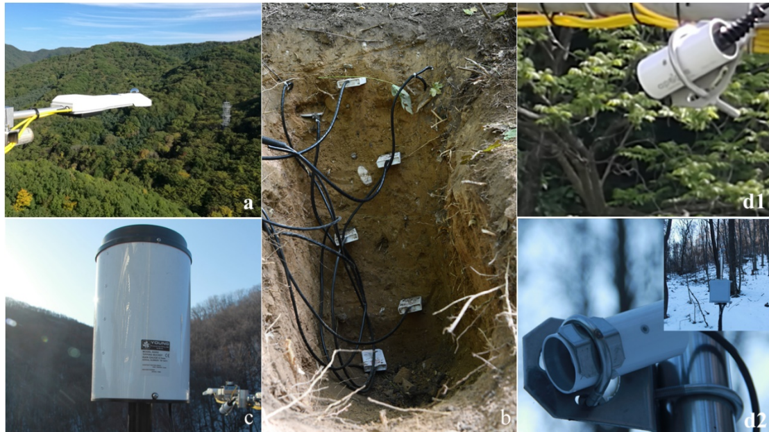
Fig. 3 Micrometeorology sensors: (a) CNR4 four-component radiometer with CNF4 ventilation and heating accessories, (b) sensor assembly for soil heat flux along with soil moisture and temperature profiles, (c) 5220 rain gage, and SI-111 infrared radiometer outside (d1) and inside (d2) forest
